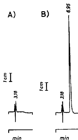
Fig. 3. (A) Chromatogram of a bovine blank plasma. (B) Chromatogram of the same bovine blank plasma spiked with TAP standard (4 mg/l). Sample pretreatment and HPLC conditions as described in the text. UV absorption at 258 nm; detector sensitivity = 0.040 a.u.f.s. Peak at t_R 6.95 = TAP.
